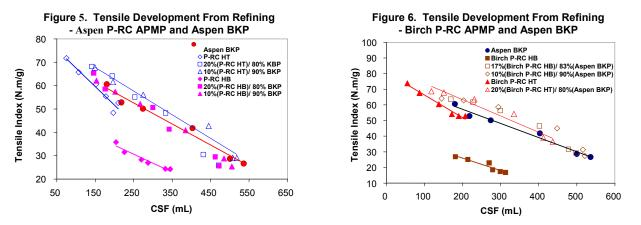
Figure 5 shows pulp tensile development from the pulp blends from the aspen. Although the aspen P-RC APMP pulps both had a lower tensile at a given freeness than the kraft pulp, the blends, after being refined to 350 ml CSF or lower, had the same, (from the high bulk, low tensile P-RC APMP HB), or even higher, (from the high tensile P-
